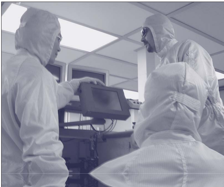
Scientists show how a screen printer can be used to produce AlphaMicon's VALiD™ liquid crystal lenses. The team wears lint-free protective clothing to preserve the dust-free, ultra-clean environment necessary for liquid crystal manufacturing. AlphaMicon, a technology start-up company, grew out of research done at Kent State's Liquid Crystal Institute. Liquid crystals are a regional strength for technology growth.
